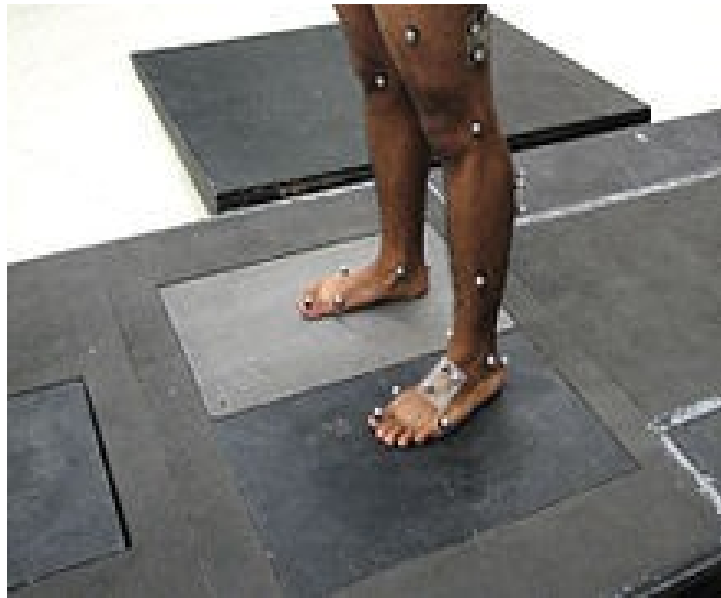
Figure 17: Two force platforms (one for each foot) used for posture and gait analysis[39]
