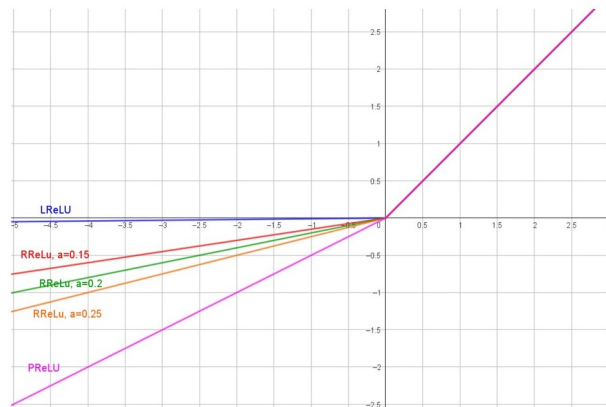
FIGURE 3.6: Rectified Linear Unit Variants.
