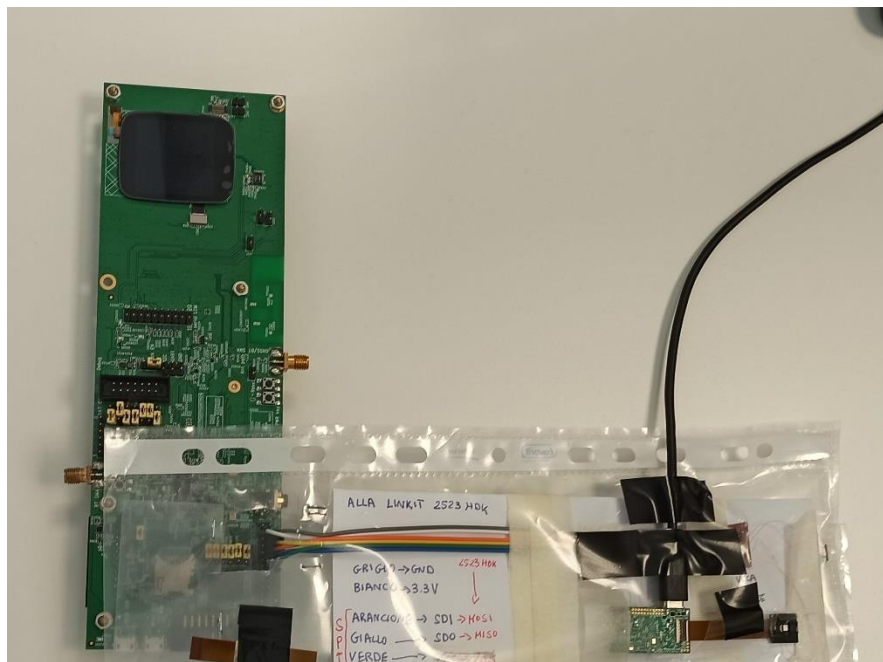
Figure 23: Developing Board of PPG sensor
