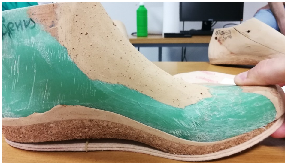
Figure 6.6: Physical comparison with the last. The physical last with the corresponding footbeds. The upper one is the Duna S.r.l. element and the lower one is the new procedure element.
