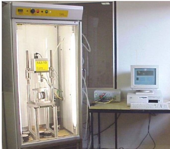
Figura 4.17 – Nottingham Asphalt Tester (NAT)
