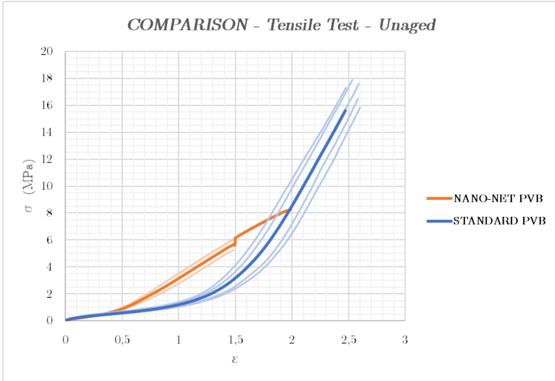
Figure 4.15 Comparison between average stress-strain diagram of unaged standard PVB and nano-net PVB
