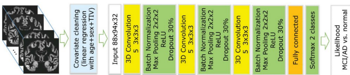
Figure 26. Convolutional neural network model layout proposed by Dyrba et al. (2020).
