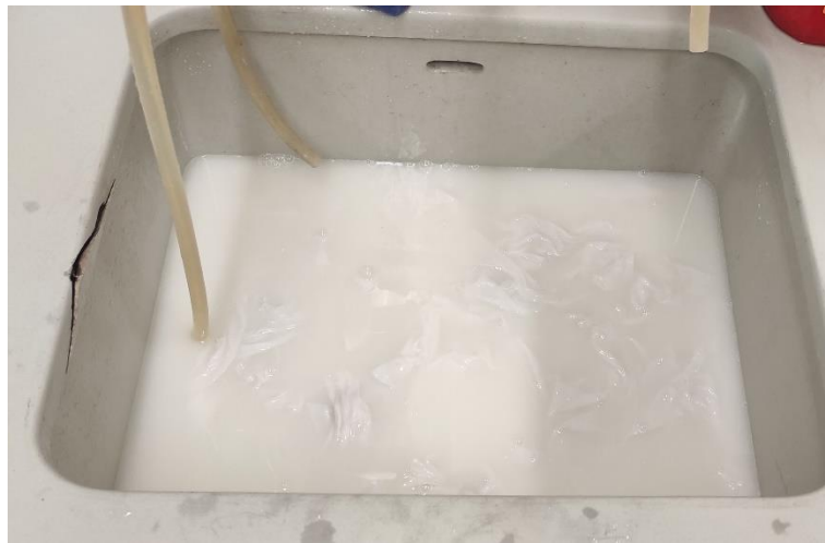
[figure 6]. Neutralization and washing of recovered Cotton textile fraction.
