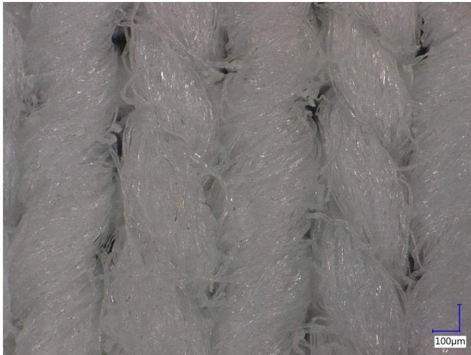
[Figure 15]. Pure Cotton treated with sodium hydroxide H_2SO_4 .
