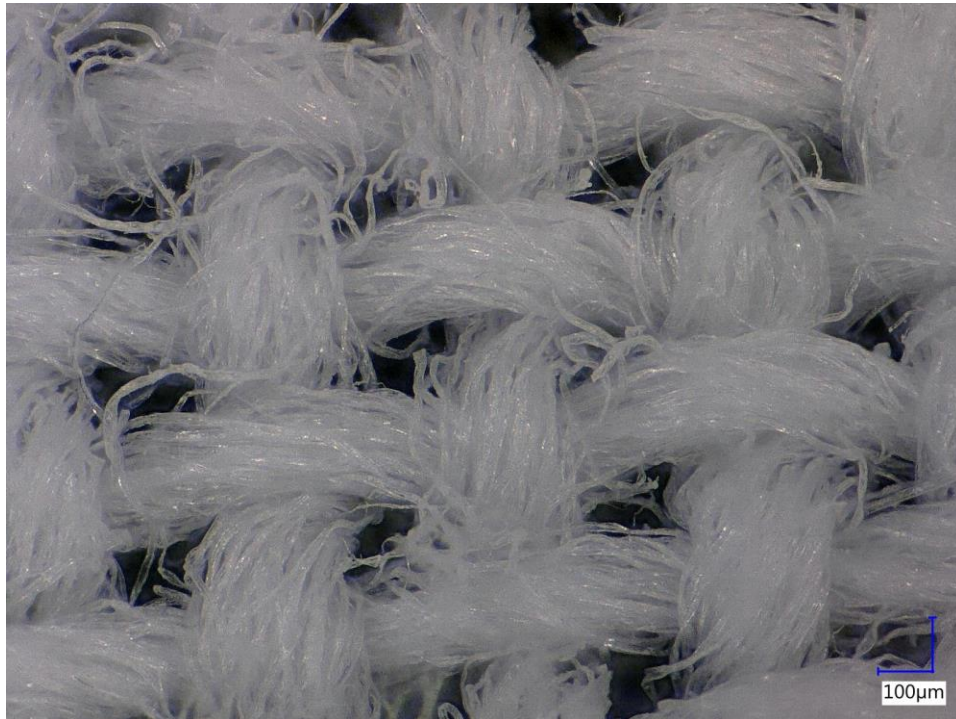
[Figure 17]. PolyCotton fiber treated with sodium hydroxide NaOH large scale.
