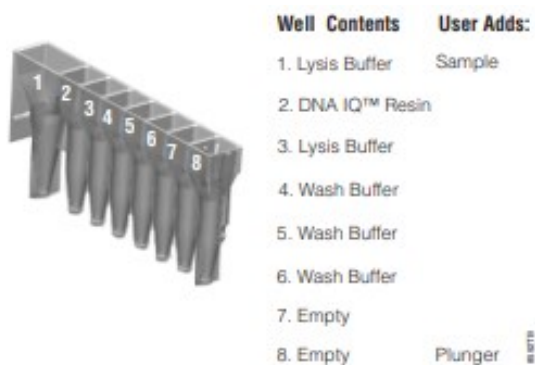
Figura 20 cartucce ready to use del kit DNA IQ™ Casework Pro Kit for Maxwell® 16.
