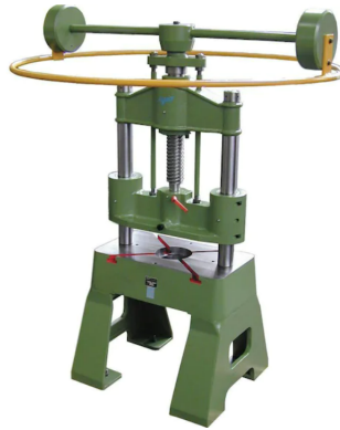
Figure 6.14: Ageo, Mechanic Press, able to produce a force of 100000 N
