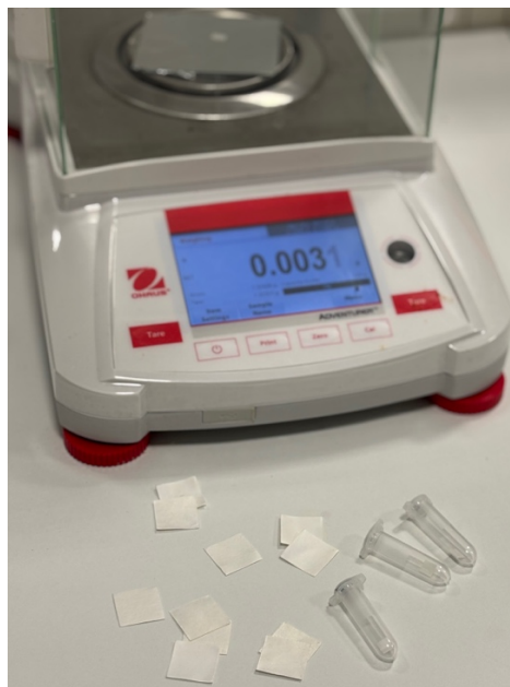
Figure 2.2 Preparation of collagen membrane specimens prior to the cross-linking procedure. The Collygen® membrane was cut into standardized square samples, individually weighed using an analytical balance.
