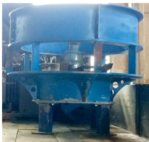
FIGURE 42: TURBINE DRAFT TUBE
