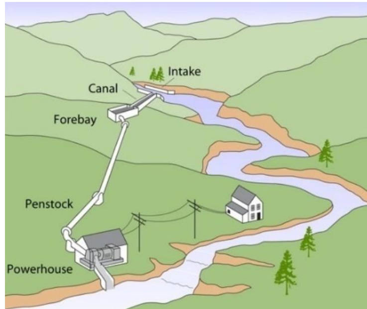
FIGURE 7: RUN-OF-RIVER SCHEMATIC REPRESENTATION (SOURCE: PICKERING, PRACTICAL SUSTAINABILITY, RUN-OF-THE-RIVER)
