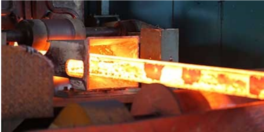
Figura 5 Scaglia superficiale http://www.siddikkardesler.com/en/index.php/production/rolling-mill
