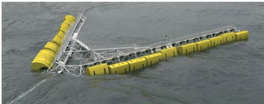
*Fig.1.18 dispositivo WEPTOS (Babarit, A. (2017). Ocean Wave Energy Conversion. Elsevier)*
