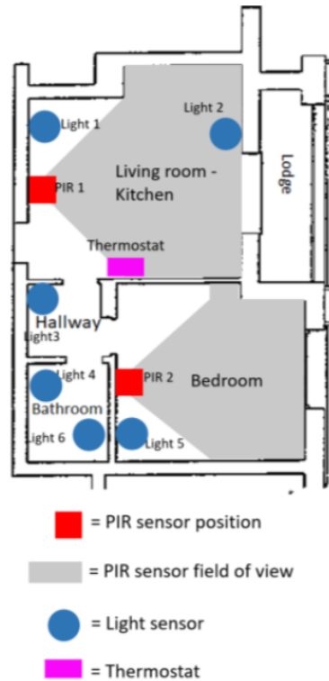
Figure 29: schematic plan of one of the apartments with installed domotic sensors.
