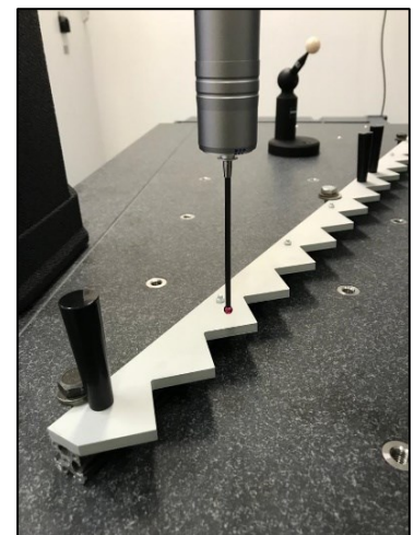
Figure 4-4. On the top, there is a 3D representation of a single calibration target. Dimensions of the single tooth of the target on the left, where there is the point obtained as the intersection given by the lines obtained from the sides of the tooth. On the right, there is a photo of the targets coupled to the CMM.
