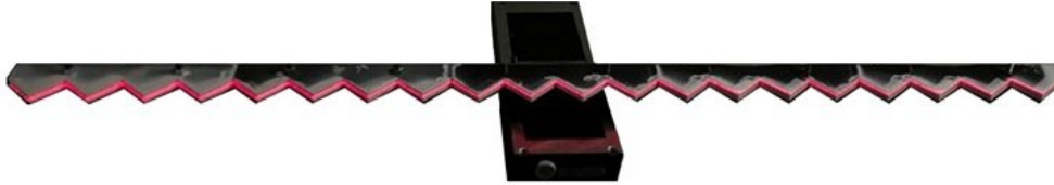
Figure 4-3. Target built with FDM process with laser beam projected.
