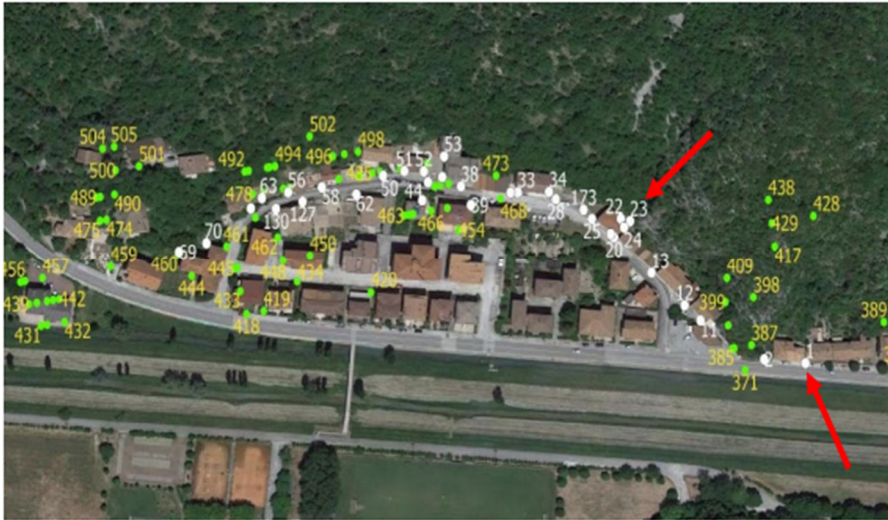
Figure 23. Map of “stable points”, in white from topographic levelling (reference points are indicated by the red arrow) and in green from DInSAR (modified from Di Stefano et al., 2022).
