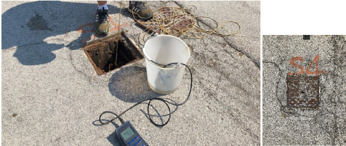
Figure 46. Setting of the diver into piezometer S4, measure of water level and electric conductivity, July 2021.
