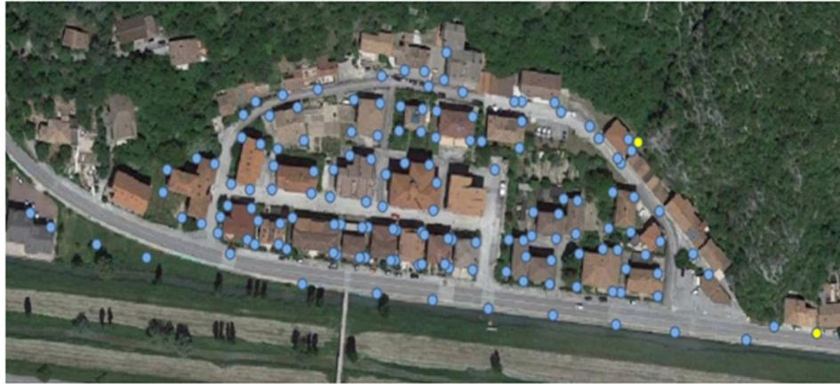
Figure 19. Targets of the topographic levelling network with identification of the two fixed markers (in yellow) (modified from Di Stefano et al., 2022).
