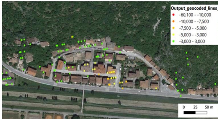
Figure 21. Deformation velocity map (processing period 2014- 2021) with the corresponding legend with 5 ranges of terrain displacement values expressed in millimetres (modified from Di Stefano et al., 2022).
