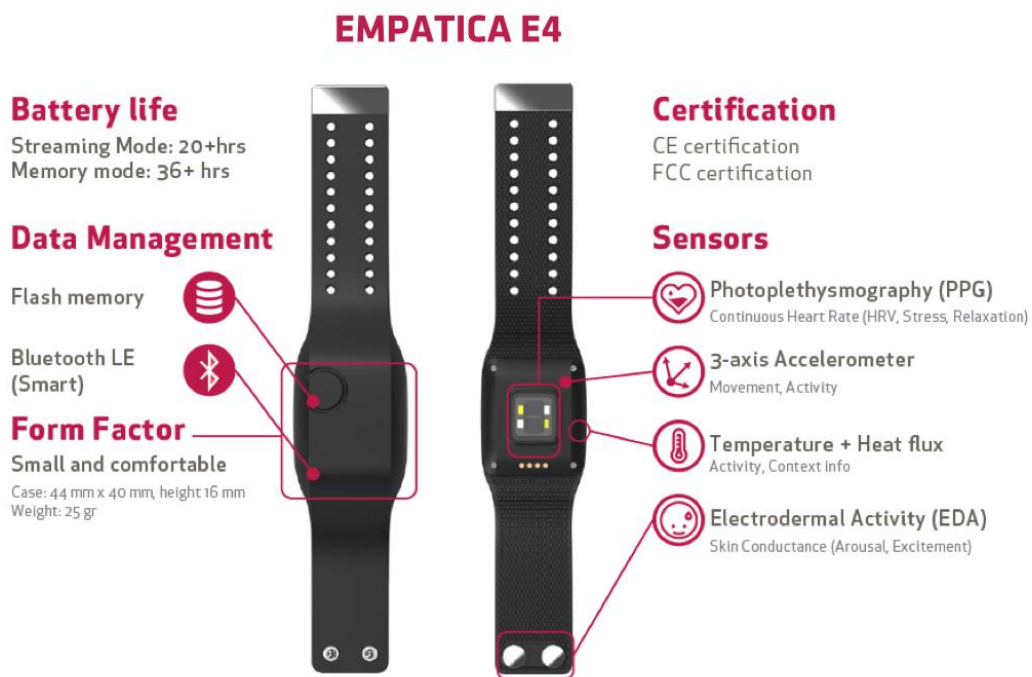
Fig. 6 Empatica E4 with the position of its sensors [41].
