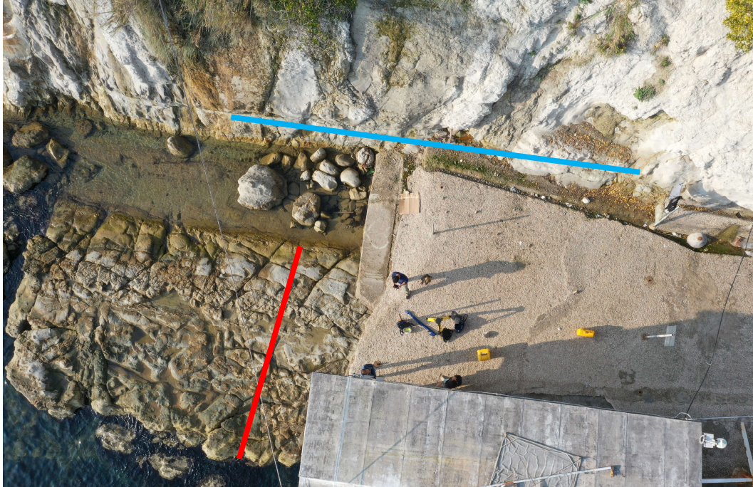
Figure 14 - Scanlines on the horizontal (red line) and vertical (blue line) portion of the cliff.
