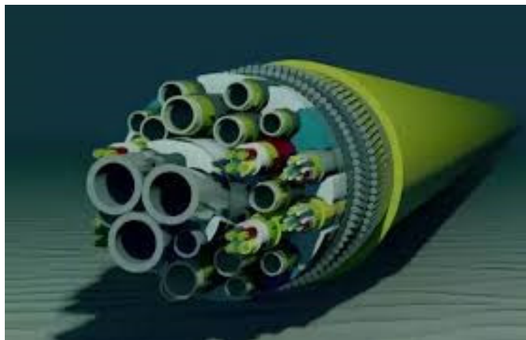
Figure 6 - Typical Subsea Umbilicals (Cross-Section)
