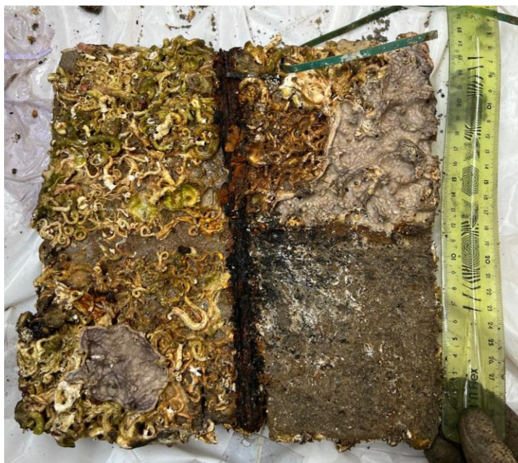
Figure 9 – Personal elaboration. Ex. photo of tile 4.1 showing the removal of the surface portion through scraping (10cm x 10cm) 16
