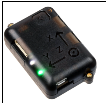
Figure 2.6: External structure of next generation IMU sensor used in the current study [78].
