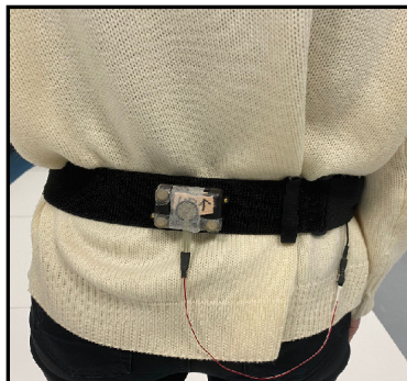
Figure 2.4: The figure illustrates the position of the force sensing resistor sensor.
