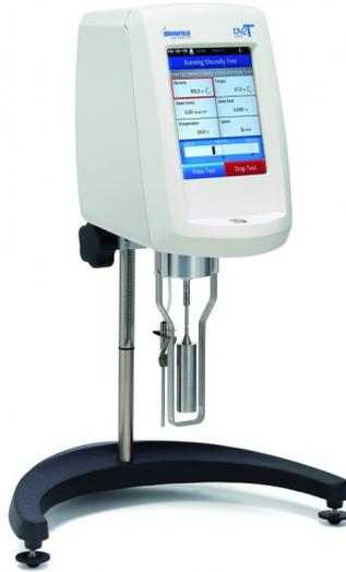
Figura 1.21: Viscosimetro Brookfield [43]
