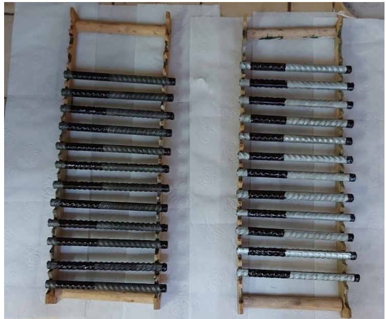
Figure.14: Resin reinforcing irons
