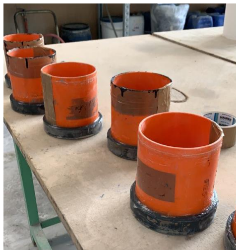
Figure.11: Cylindrical specimen formwork
