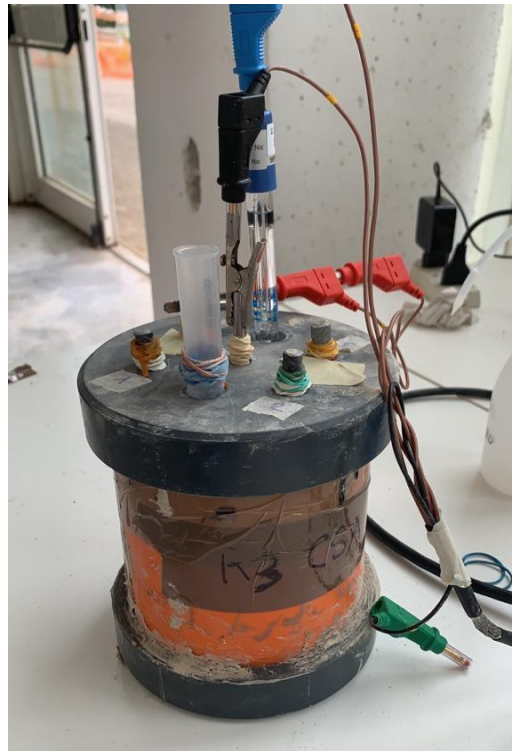
Figure.23: Instrumentation used for corrosion testing and connections with the specimen to be tested.
