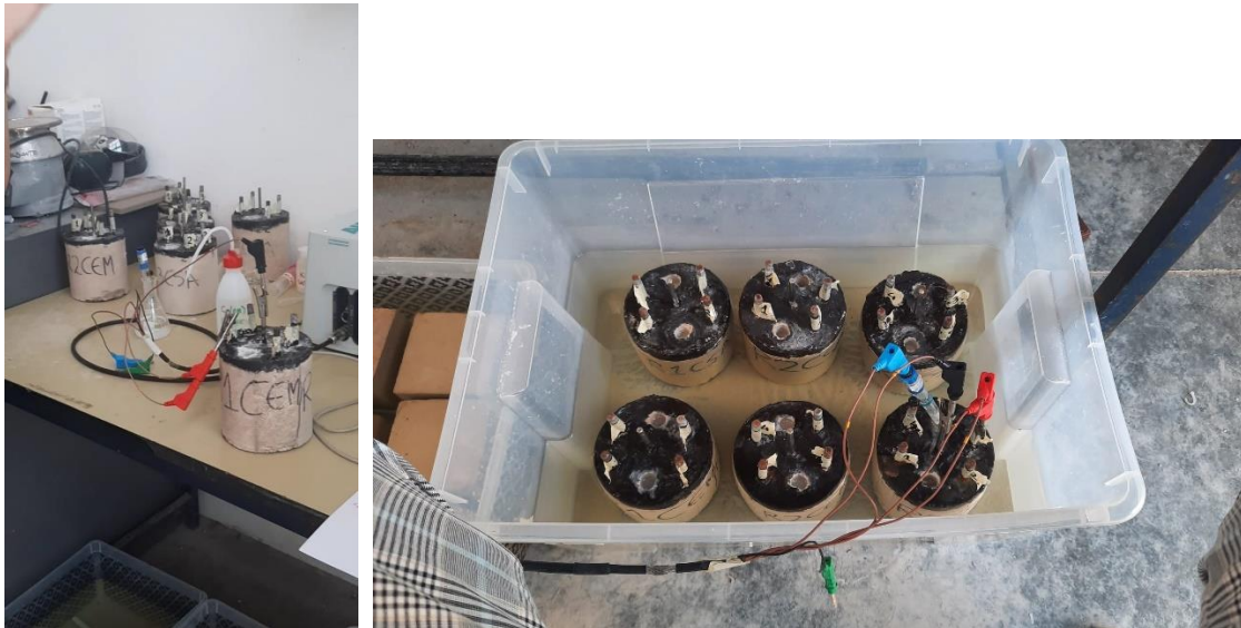
Figure.33: wet and dry potential measurements
