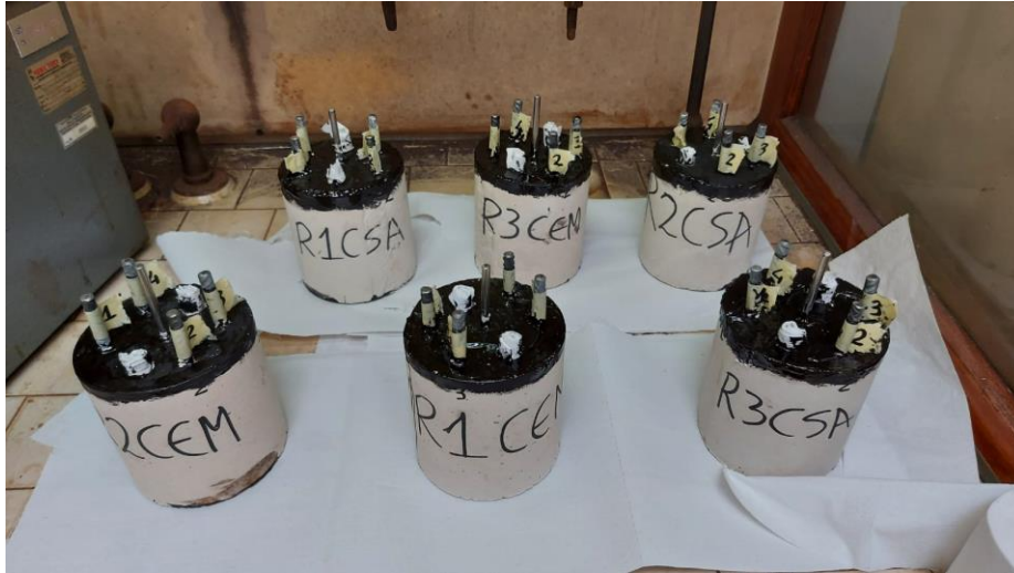
Figure.31: Specimens after resin coating
