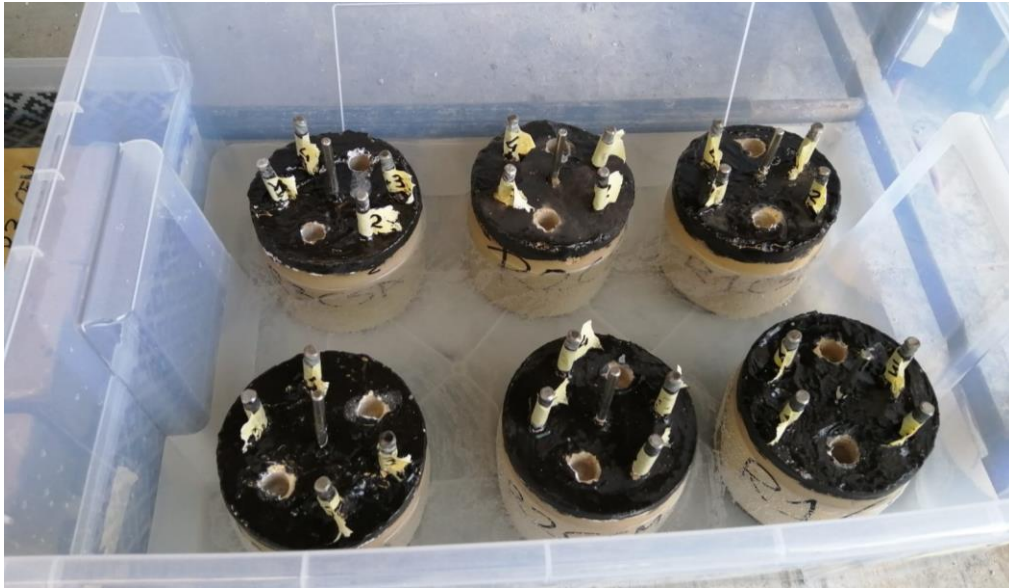
Figure.32: Specimens in 3.5% NaCl aqueous solution.
