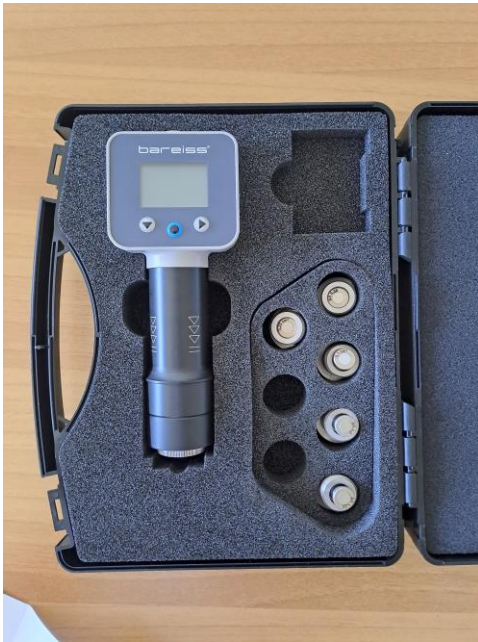
Figura 11 - BAREISS HPE III BASIC Shore D.
