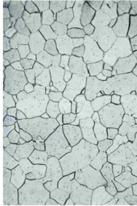
Fig.4.6a Ferrite e perlite,
