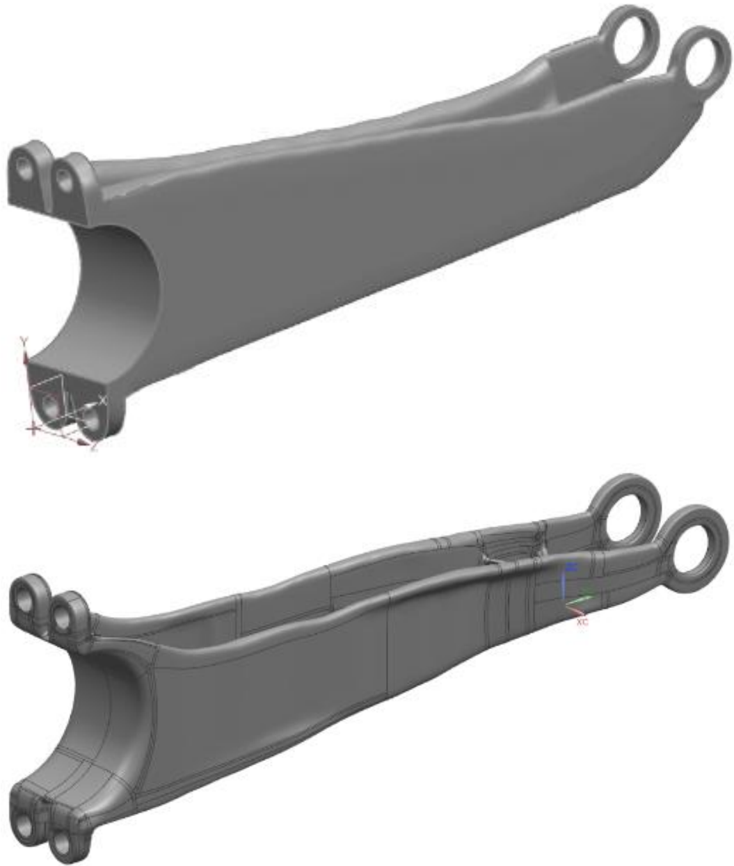
Figura 6.12: Generative Design Casting in NX e Solid Edge
