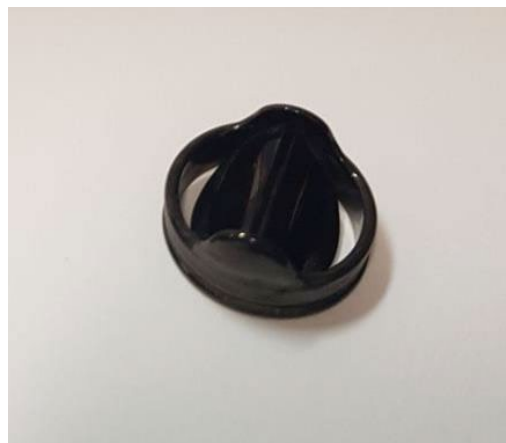
Figure 18:Aortic valve used in this test bench.
