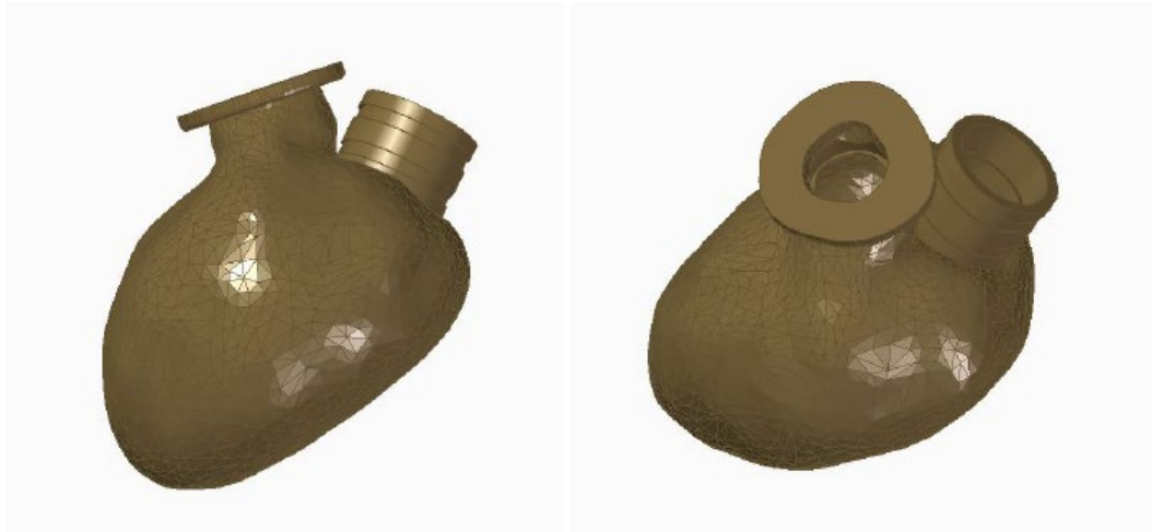
Figure 17: 3D- printed Left Ventricle
