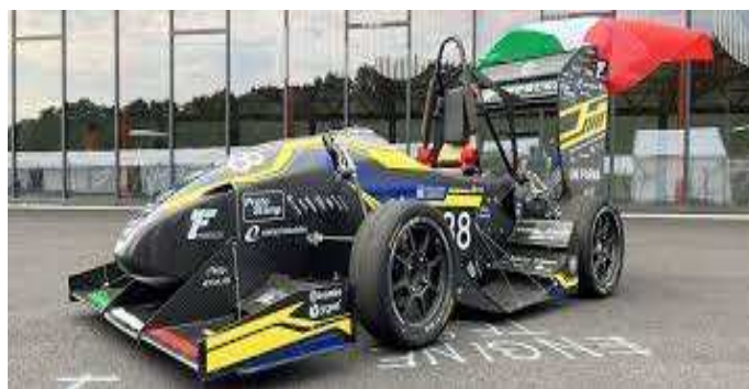
Figura 1.17: Formula SAE con sidepods alari
