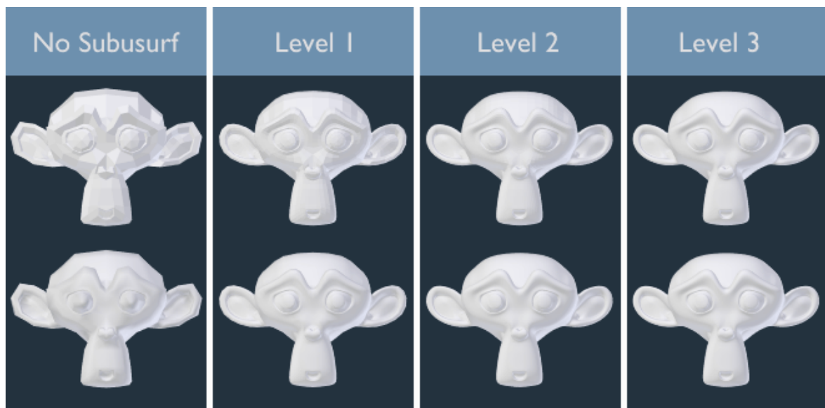
Figura 2-12: Effetto del Subdivision Surface Modifier flat shaded (sopra) e smooth shaded (sotto) [10]
