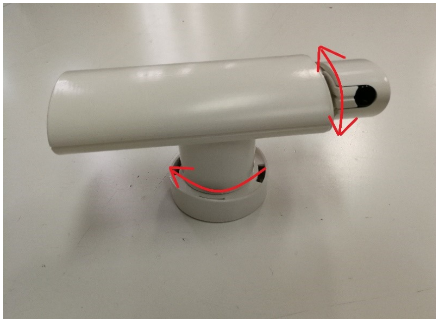
Figura 16-Ceiling Node (Scanner IR)
