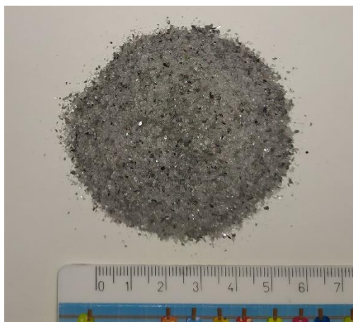
Figura 3.2 – LCD macinato \varnothing < 1\text{mm}
