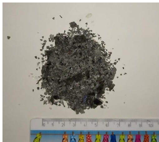
Figura 3.3 – LCD macinato \varnothing > 1\text{mm}
