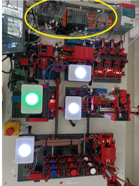
Fig. 4.6: A yellow balloon highlights the B&R control system in a sight from above
