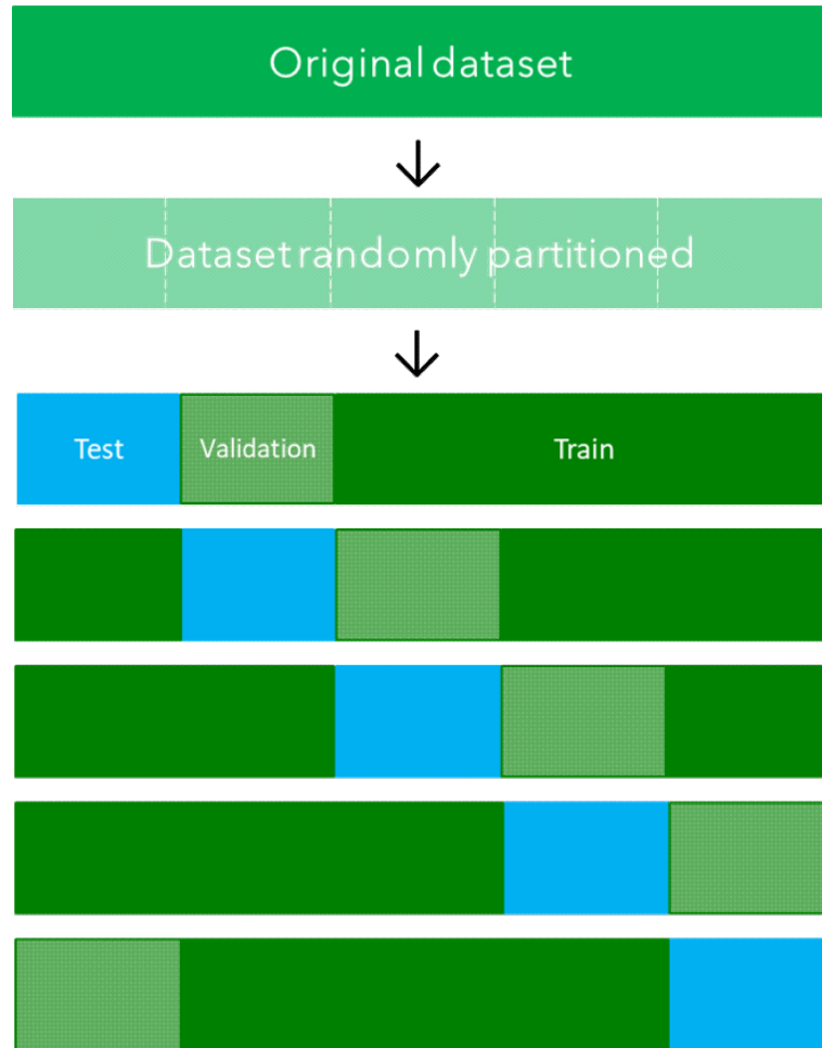
Figure 4.1: A schematic illustration of K -fold cross-validation for K = 5 . The original dataset (shown in dark green) is randomly partitioned into K disjoint sets (shown in light green). Then, for each subset, K-1 parts are used for training the model (shown in green), one of which is used for validation (shown in light green) and the remaining part is used for testing (shown in blue). This process is repeated K times for all possible choices of the test set, producing test errors. The final performance is reported by averaging the errors from each iteration.
