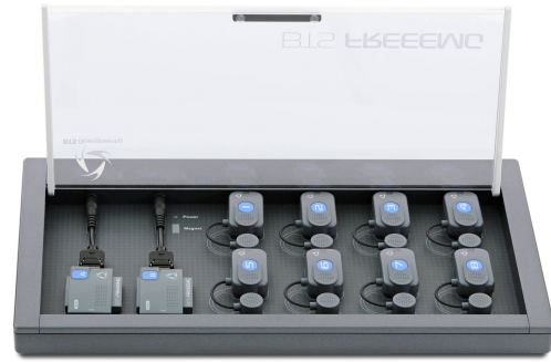
Figure 17: Charging box BTS electrodes. When batteries are completely charged, electrodes guarantee up to 6 hours of nonstop acquisition.
