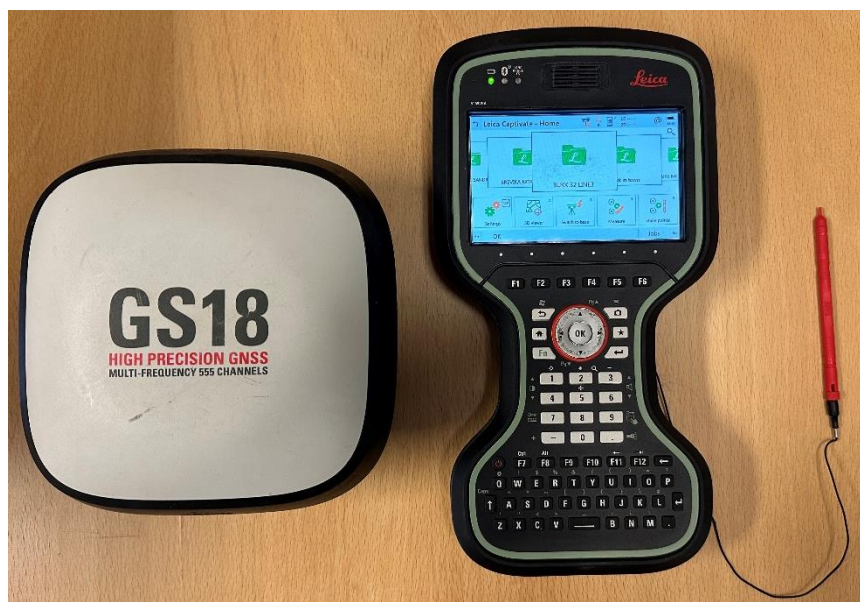
Figure 9.1 Leica dGPS used to survey the cableway post structures during fieldwork.
