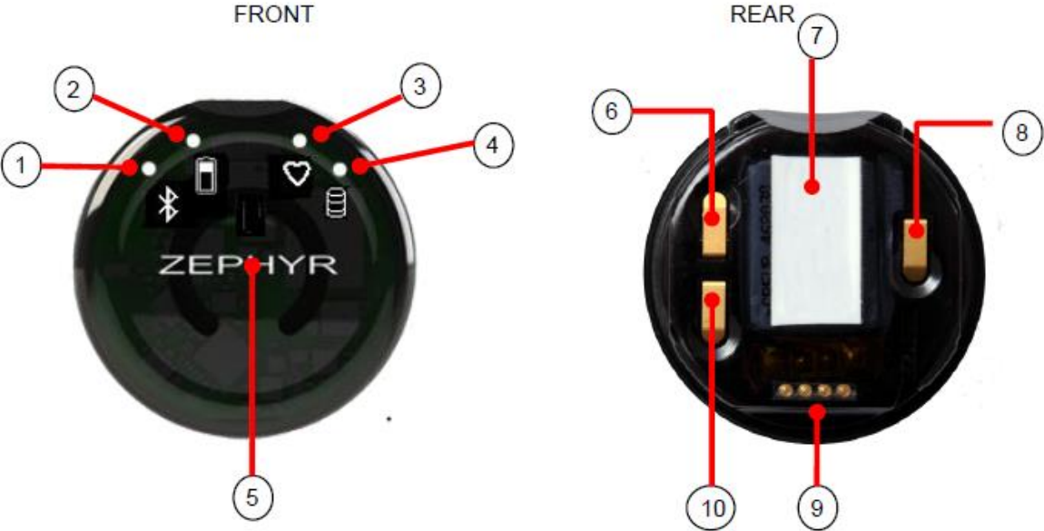
Figure 8.2 – BioHarness Module, front and rear. 1 is the blue Bluetooth indicator LED, 2 is the orange battery indicator LED, 3 is the red HR detection status LED, 4 is the green logging indicator LED, 5 is the ON/OFF button, 6 is the ground spring contact, 7 is the rear label location, 8 is the ECG signal spring contact, 9 is the USB charging/configuration contacts, 10 is the breathing signal spring contact.
