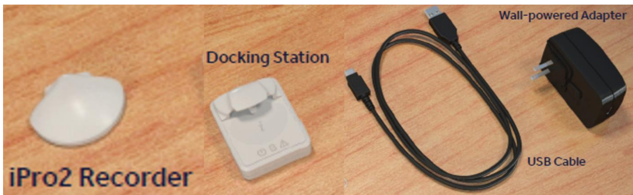
Figure 8.6 – The components required for charging the iPro2 CGM: the iPro2 Recorder, the docking station, the USB cable, and the wall powered adapter.
