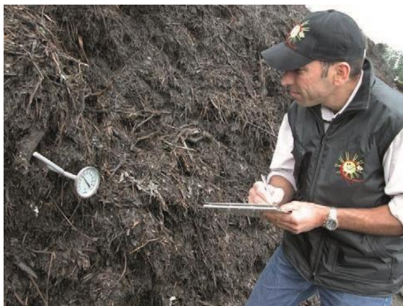
Slika 2: Temperature measurement is important to control the composting process.
