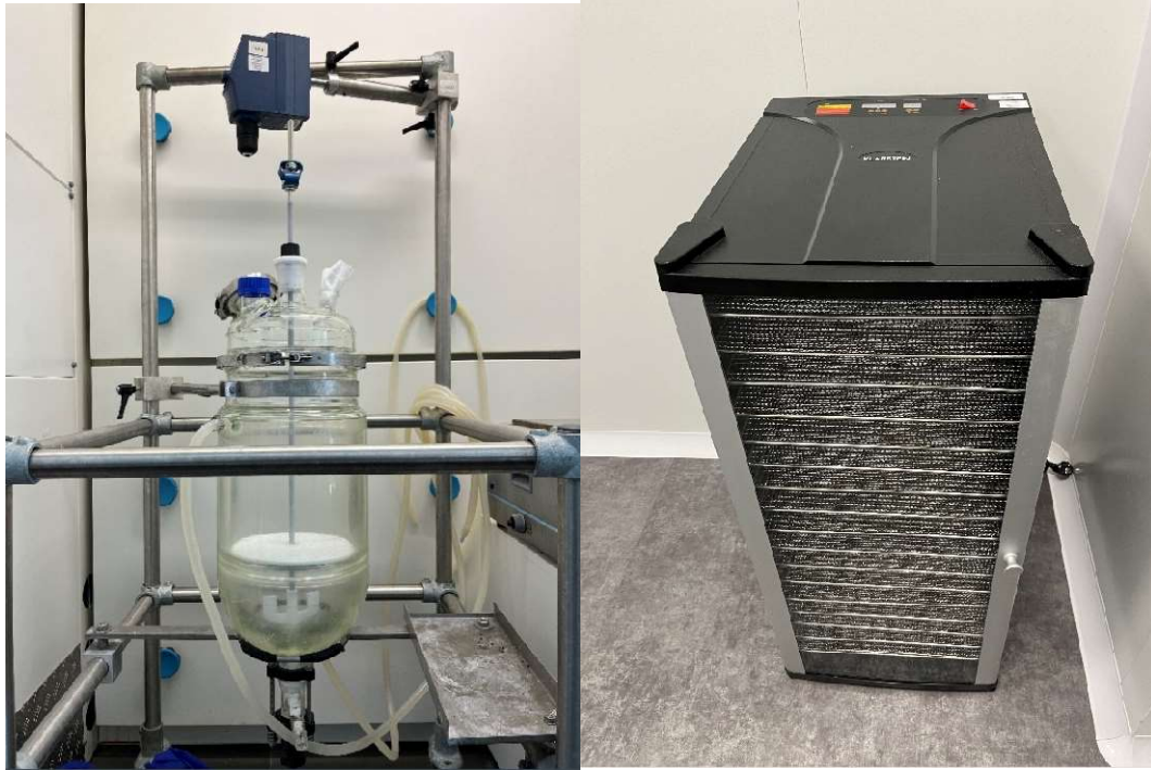
FIGURE 17 IN THE LEFT PICTURE THERE IS THE REACTOR, IN THE RIGHT ONE THERE IS THE OVEN
