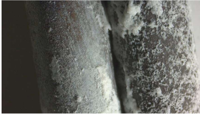
FIGURE 40 RESULT OF THE 9° TEST: COATING SHOWN OVER THE BAR WITHOUT OXIDE LAYER (ON THE LEFT) AND COATING SHOWN OVER THE BAR WITH THE OXIDE LAYER (ON THE RIGHT)
