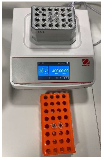
FIGURE 31 TEST TUBES WITH P AND M SAMPLES READY TO BE PLACED IN THE SHAKER
