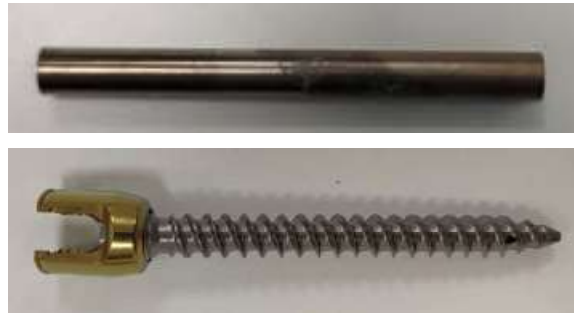
FIGURE 20 GRADE 6 TITANIUM BAR (ON THE TOP), GRADE 4 TITANIUM SCREW (ON THE BOTTOM)
