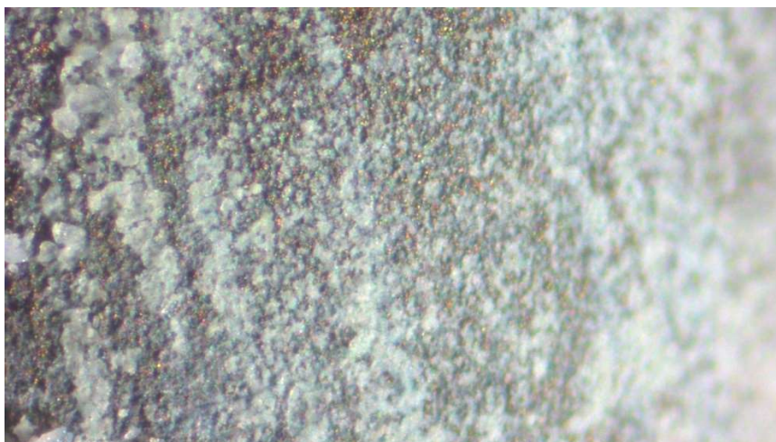
FIGURE 50 A HOMOGENEOUS AND STRONG RECOATING ON THE BAR, ANALYZED THROUGH A MICROSCOPE, WAS OBSERVED AFTER IT UNDERWENT THE PROCEDURE DESCRIBED IN EXPERIMENT 5
