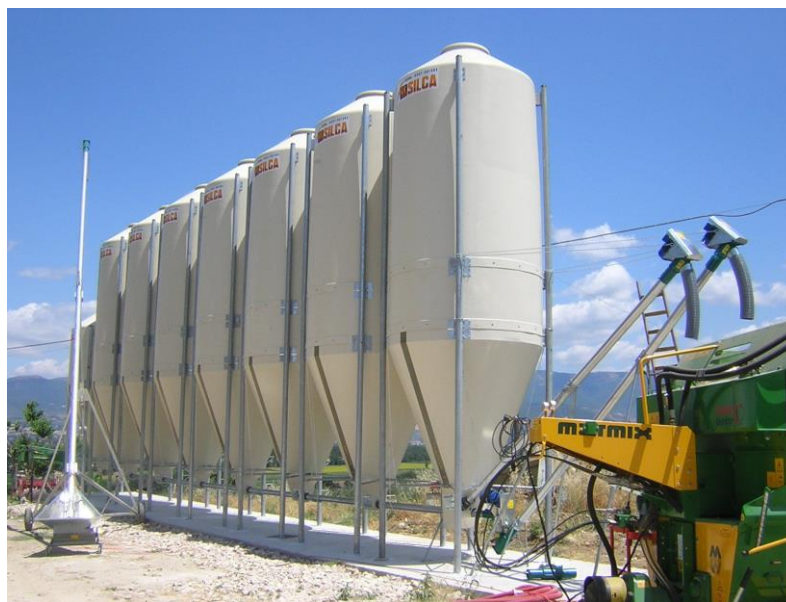
Figura 16 – Silos in vetroresina (silosilca.it)
