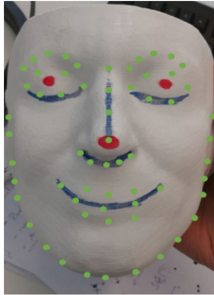
Figure 16 Facial landmarks (in green) detected over a phantom head.
