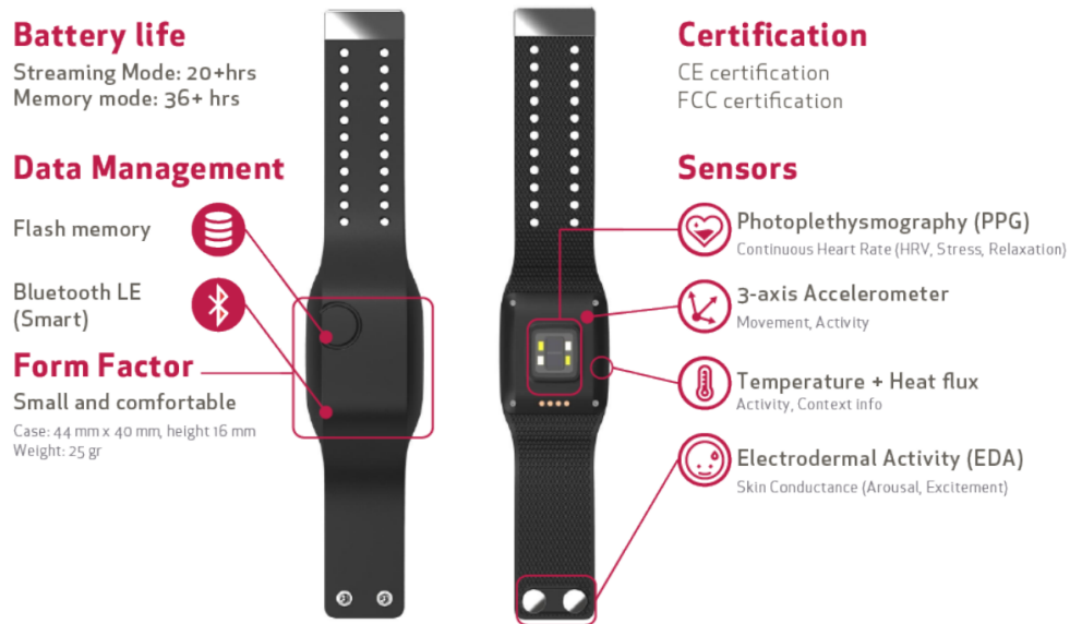
Figure 5.1: Empatica E4 with the position of its sensors [67].
