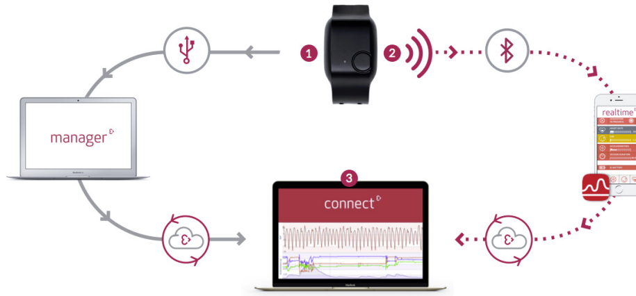
Figure 5.3: Empatica E4 Working Modes [67].
