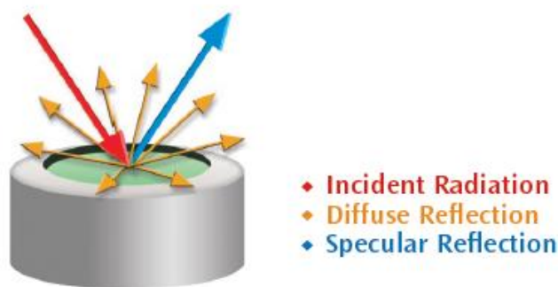
Figure 2 The two-reflection mechanisms occurring when light is incident on a material. Taken from [24].
