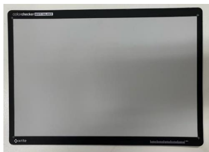
Figure 17 White standard of known reflectance used for the calibration of the white.
