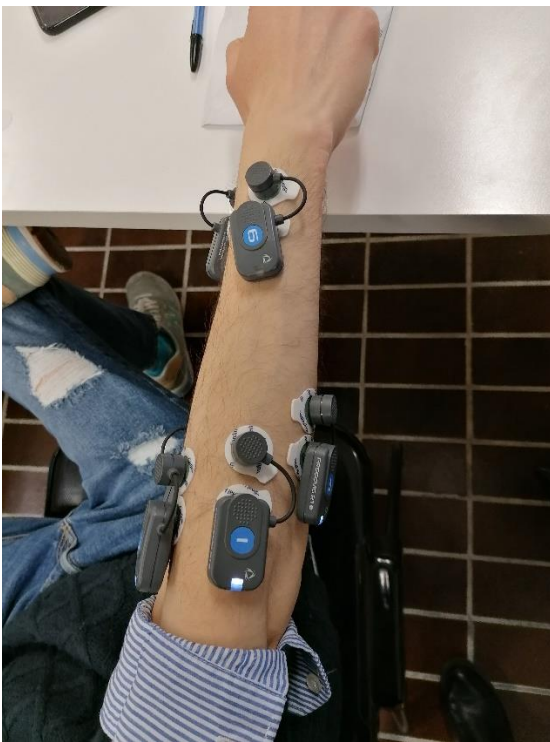
Figure 5: a) Setup of the electrodes adopted for handwriting recognition task. On the left, posterior view of the right arm; on the right, anterior view. b) Right arm of one subject after the placement of the electrodes.
