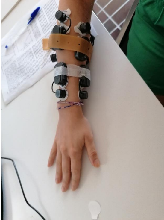
Figure 6: Setup of the electrodes, further fixed using medical adhesive tape and tourniquets, in order to lock the electrodes in their correct position during motion.
