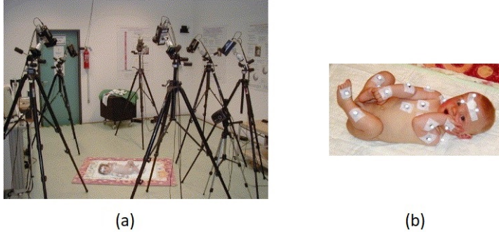
Figure 2.2: Representation of the tracking system presented by Meinecke et al. [27] (2006). In picture (a) is shown a photo of the 7 cameras positioned around the preterm infant. In figure (b) are shown the markers positioned on the body of the preterm infant.
