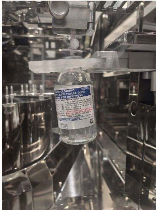
Figure 4.4. Forced insertion of the mini-spike into the 100ml vial. A tilt is visible.
