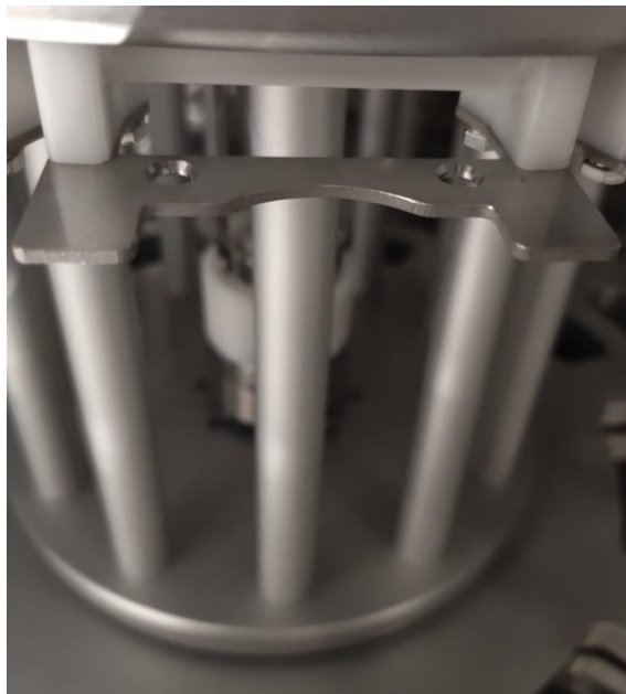
Figure 3.2. Representation of vial clamp housing in the carousel.
