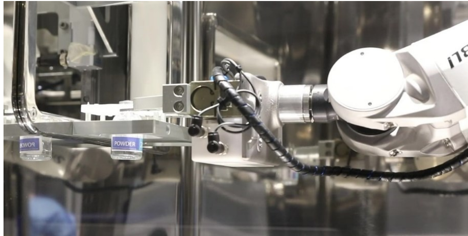
Figure 3.5. Representation of vial clamp housing on station communicating both with anthropomorphic and cartesian robots.
