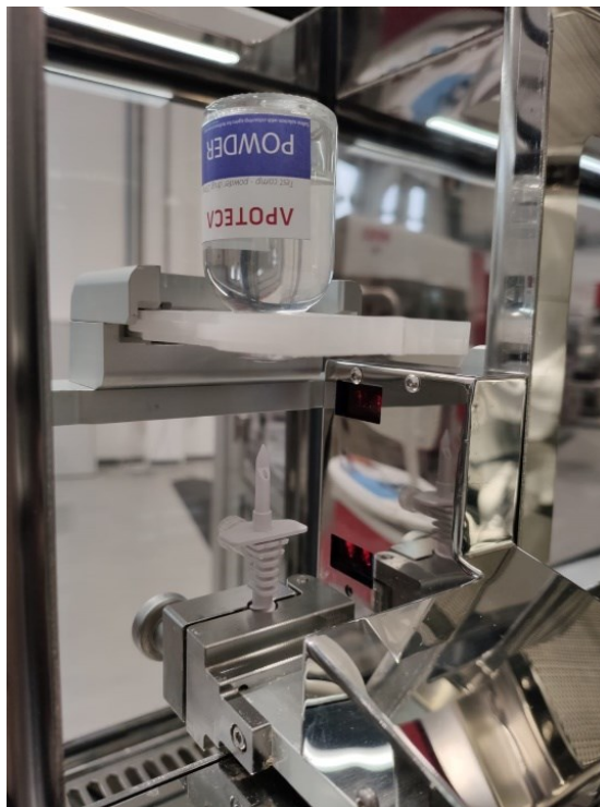
Figure 3.3. Representation of vial clamp housing in the dosage area.
